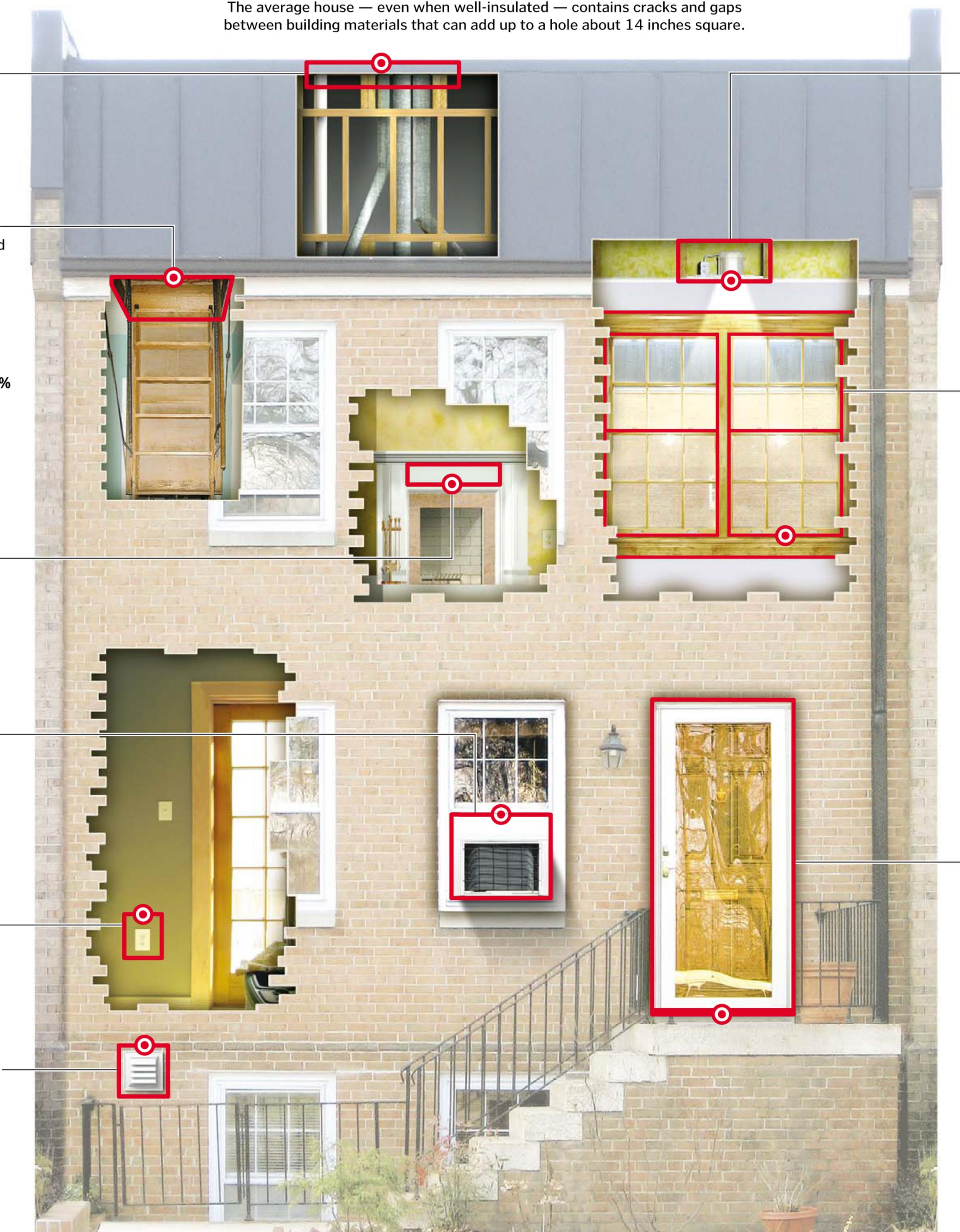
Recessed lights, wiring and **plumbing** in insulated ceilings can result in heat loss. Hightemperature, flexible caulk can be used to fill gaps.
